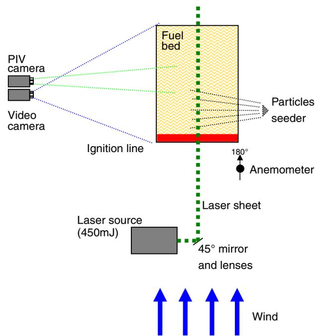
**Fig. 2** Schematic of the experimental device
